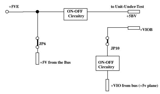
As you can see, there will be a conflict in case the external supply is connected while the jumper is still in place. This circuit is repeated for each of the 4 voltages.
